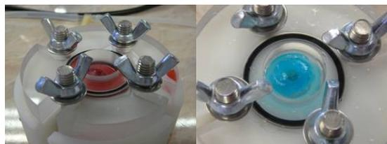
Figure 1 – Burst Pressure Test Rig
