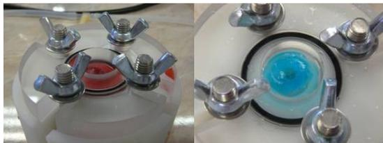
Figure 1 – Burst Pressure Test Rig
